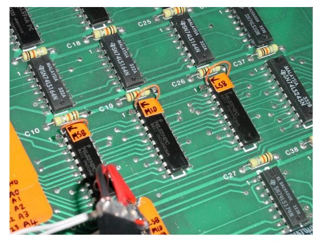
5. Solder the 2 wire power cable to each side of the resistor above the 74LS138 at A1.
