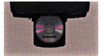
Two-Way Disc Tray opening: Full size tray for LDs and small size tray for CDs.
